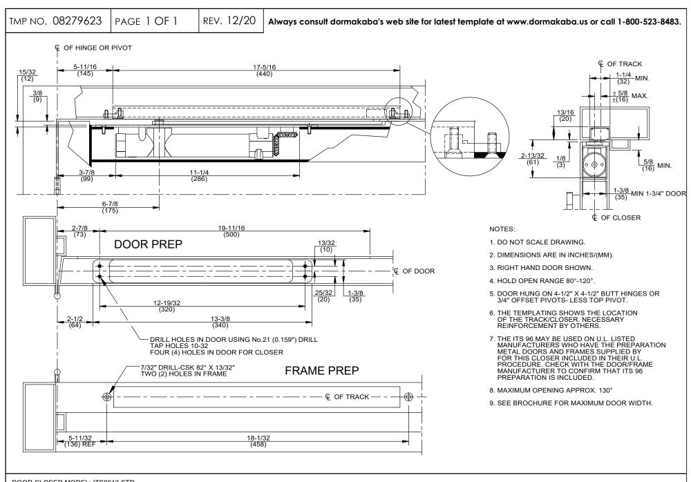
DOOR CLOSER MODEL: ITS9613 STD CLOSER IN DOOR TRACK IN FRAME WITH ACCESSORY TRACK BRACKETS (METAL DOOR AND FRAME)
